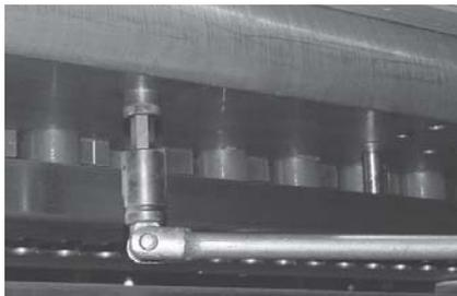
7. Lower die shoe onto steel rods and remove the bottle jacks.
