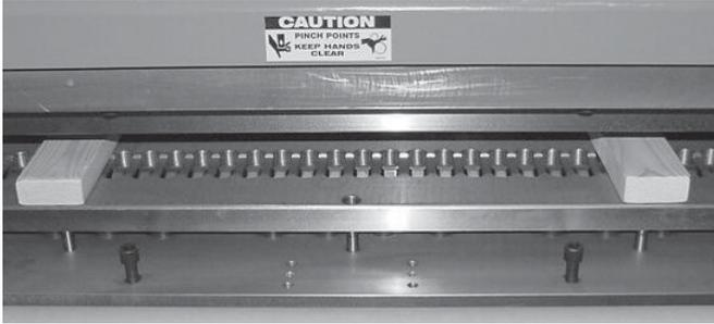
4. Using two bottle jacks and two brackets similar to those shown, jack both ends of the lower die until
