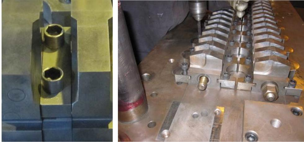
6. If the center spacer was removed it must be aligned with a square and bolted in place to reassemble the die. Please refer to the picture below showing the starter spacer being aligned with a square.
