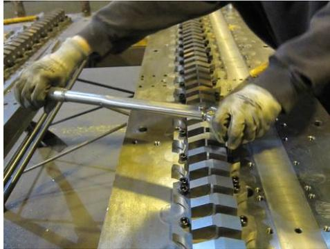
16. After sharp edges are restored, and the punches have been assembled to the die shoes, examine all urethane stripper springs for signs of rupture and excess deflection. If any show rupture cracks or have an overall relaxed length of less than 1 7/8" (48 mm), discard them and replace.
