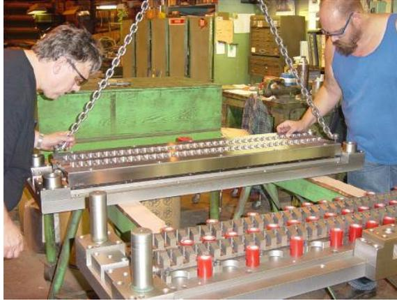
3. Remove the urethane springs and clean the die. Replace the urethane springs if they are cracked or damaged, or have been compressed to a height of  $1 \frac{7}{8}$ " (48 mm) or less.
