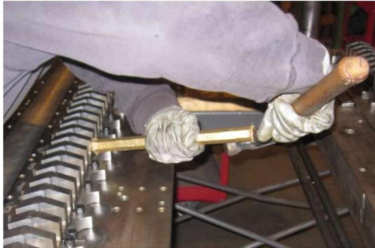
13. Next assemble upper die in much the same way the lower die was assembled, minus the starter spacer details. After the punches and spacers have been assembled in the proper order and tie rod and clamps installed and snugged, the two die halves are ready to be put back together to begin the final punch alignment process.
