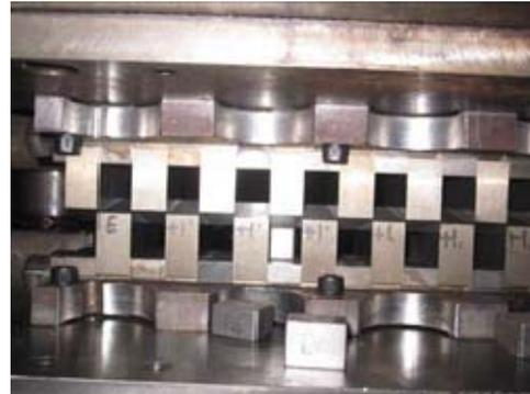
15. After bumping the punches, ***torque the hold down clamps to 32 ft-lb (44 N-m)***. Check the punches to make sure that they didn't move during the torquing process. This is best done by assembling the die again and closing the die until the punches engage each other. If any of the punches moved bump as required to attain the proper clearance.
