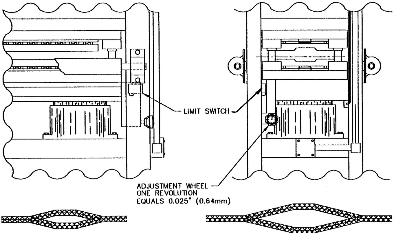
In this case, the stitch is incomplete. Turn the adjustment wheel counter-clockwise to make a deeper stitch.
