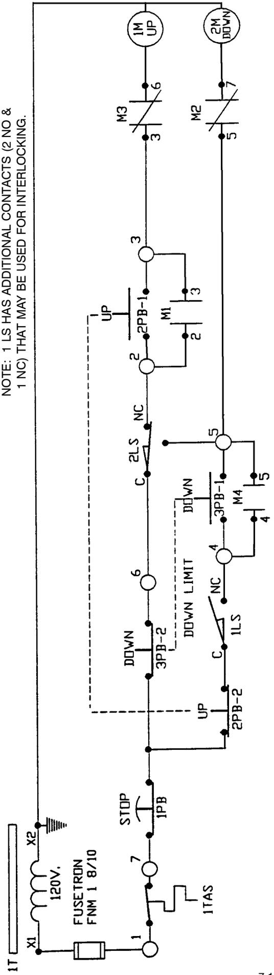
NOTE: 1 LS HAS ADDITIONAL CONTACTS (2 NO & 1 NC) THAT MAY BE USED FOR INTERLOCKING.
