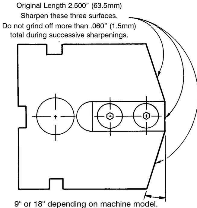
reassembled and placed back into the machine. The die and press each have a marking labeled "Front". The die is symmetrical, but it should be placed back in the press as originally assembled. If grinding equipment is not available to sharpen teeth as a unit, they may be ground individually. Read the instructions for the procedure to remove and replace teeth.
